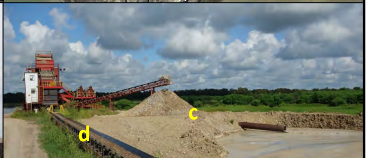
Representative view of proposed dewatering and redeposition/discharge (c) of unmarketable sediments (e.g., fine sand, silt and clay) back into mining pits at a dewatering/de-sanding plant (b). Marketable sediments will then be transported to the existing processing plant via a conveyor belt system (d).
