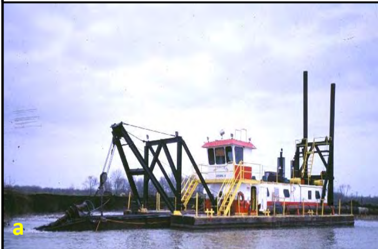
View of the stripping dredge boat to be used to remove overburden.
