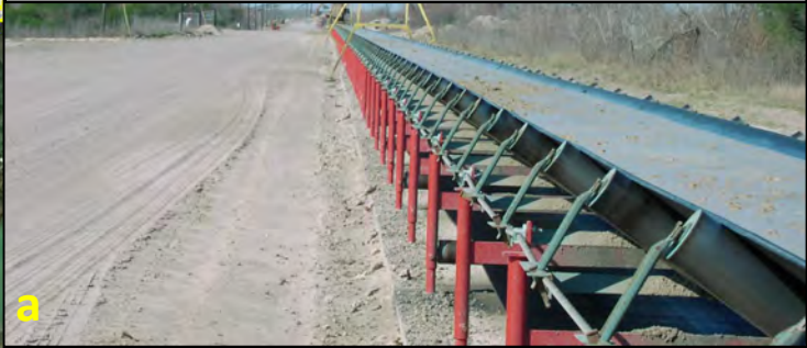
Representative view of existing and proposed conveyor belt system (i.e., belt line, access road, and power supply) (a) to be used to transport the marketable sediments to the existing processing plant (b).
