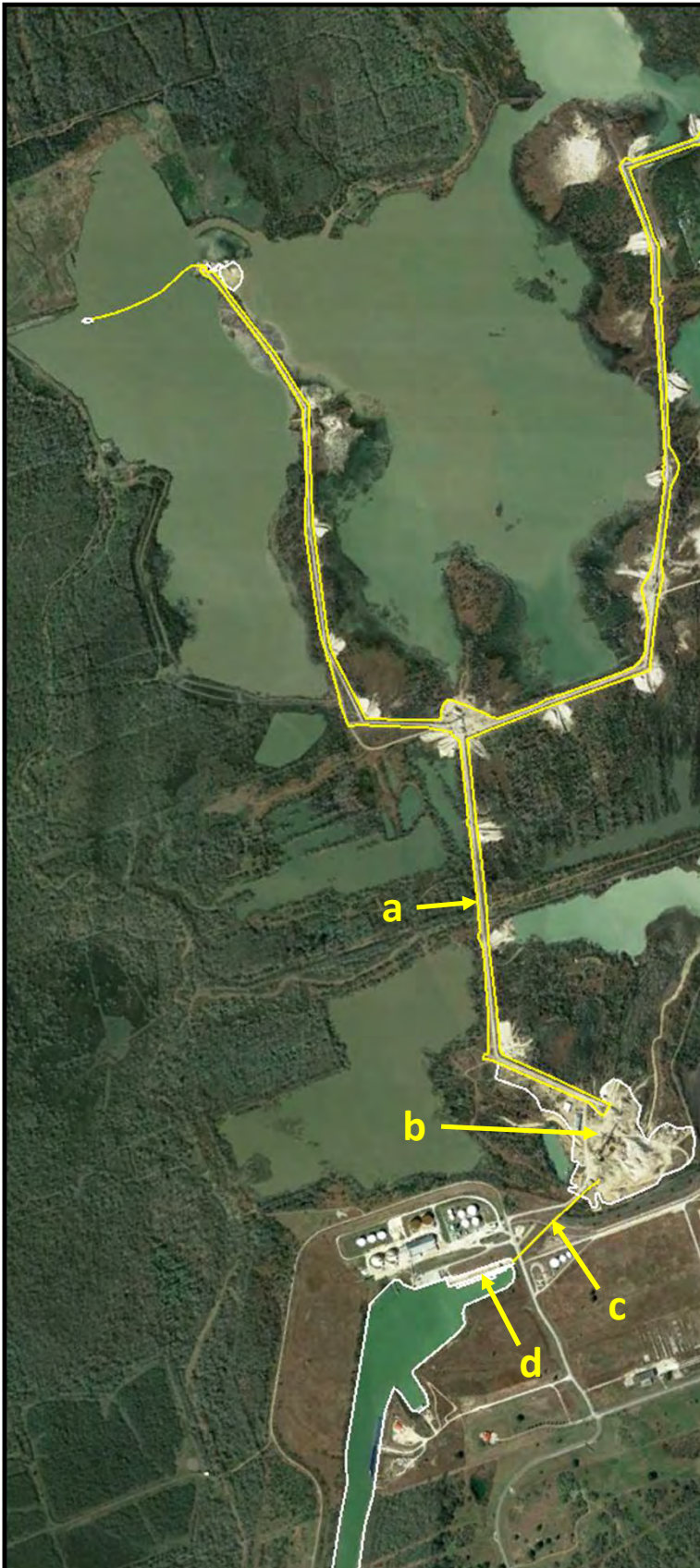
Aerial view of existing Fordyce infrastructure (i.e., conveyor belt system (a & c), processing plant (b), and barge dock (d)) to be used to transport, process, and deliver finished material.
