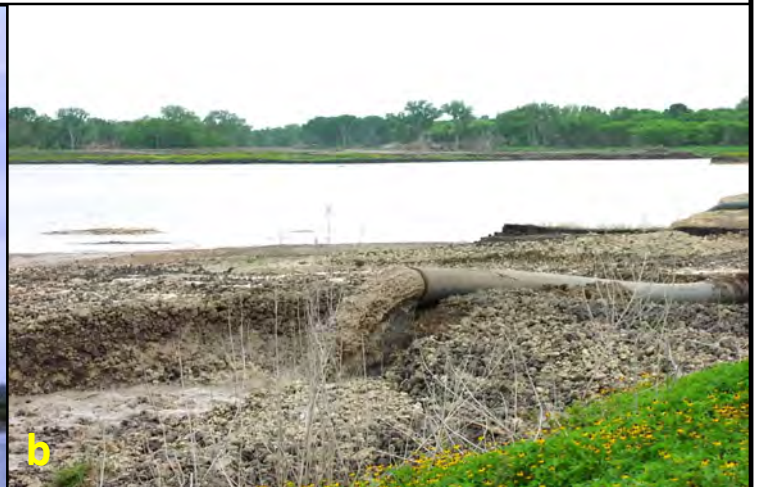
Representative view of proposed redeposition/discharge of overburden back into mining pits.
