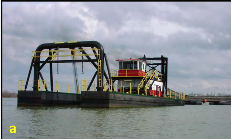
View of production dredge boat (a) to be used to dredge 25 to 40 feet of marketable sediments. The slurry will then be pumped to a dewatering/de-sanding plant (b).
