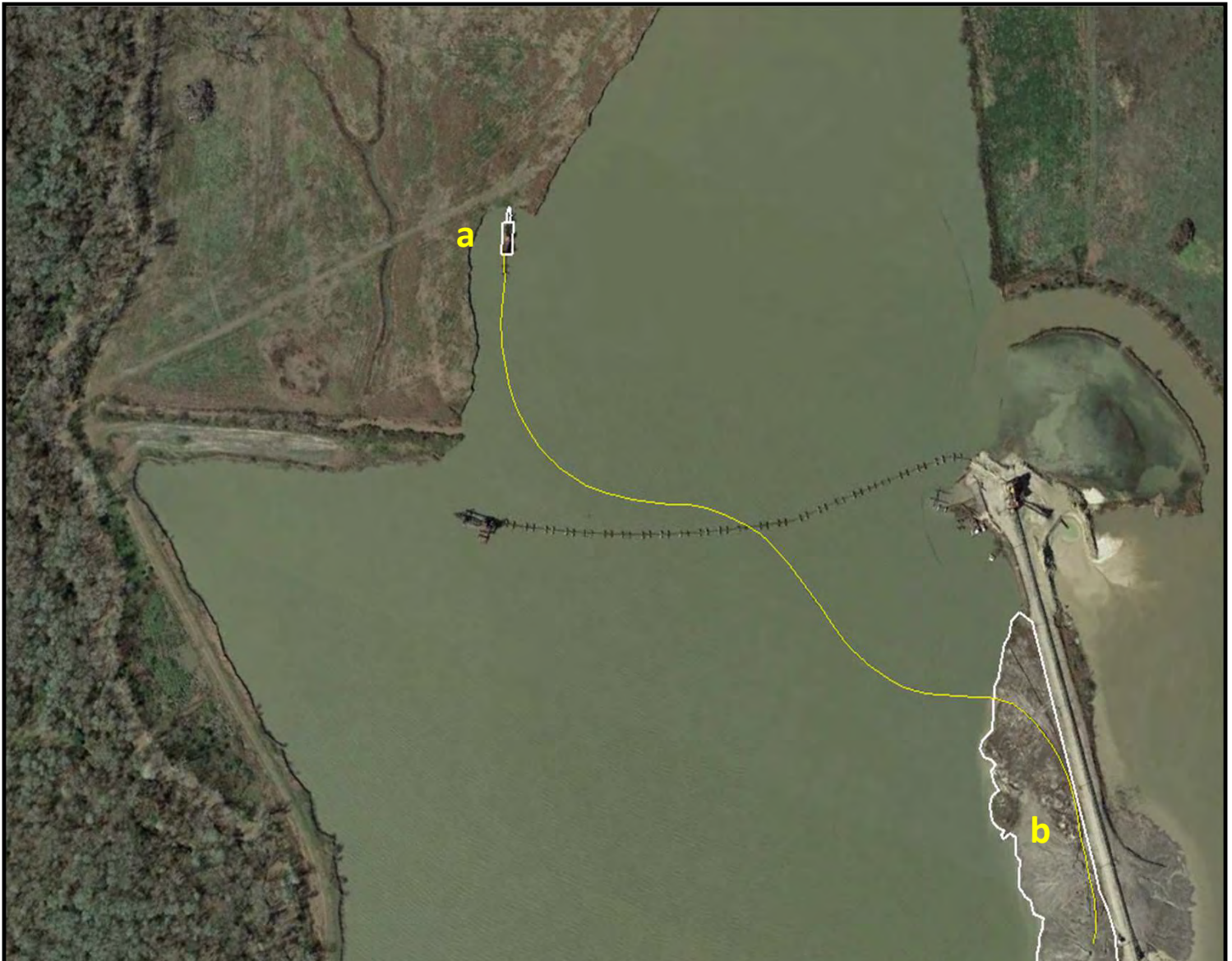
Representative aerial view of proposed overburden removal stage. During this stage, a stripping hydraulic dredge (a) will remove 12 to 15 feet of overburden and redeposit/discharge the overburden (b) back into mining pits near areas that are being dredged/mined.
