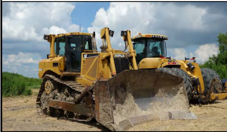
Representative bulldozers, scarpers, and similar heavy equipment to be used to clear and level the land to be mined next.
